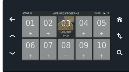
If the door has been opened because portions have been **removed**, touch the relevant tray (for example, 03), and set the number of portions removed using the "-" button (in the example, 4 portions have been removed therefore go from 10 to 6).
